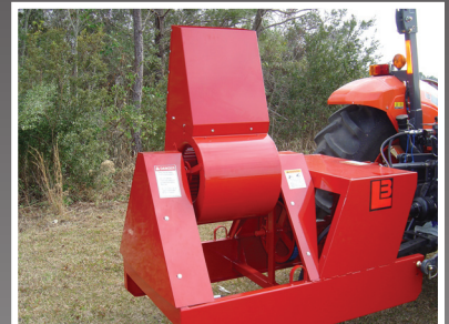
THE POULTRY HOUSE BLOWER
