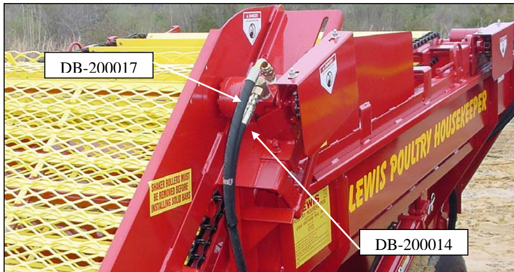
Loading Motor Hoses
