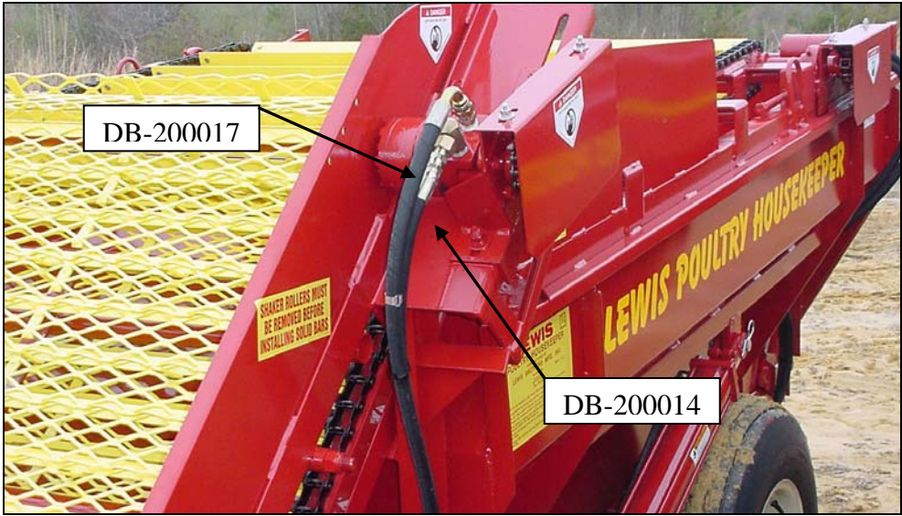
Loading Motor Hoses
