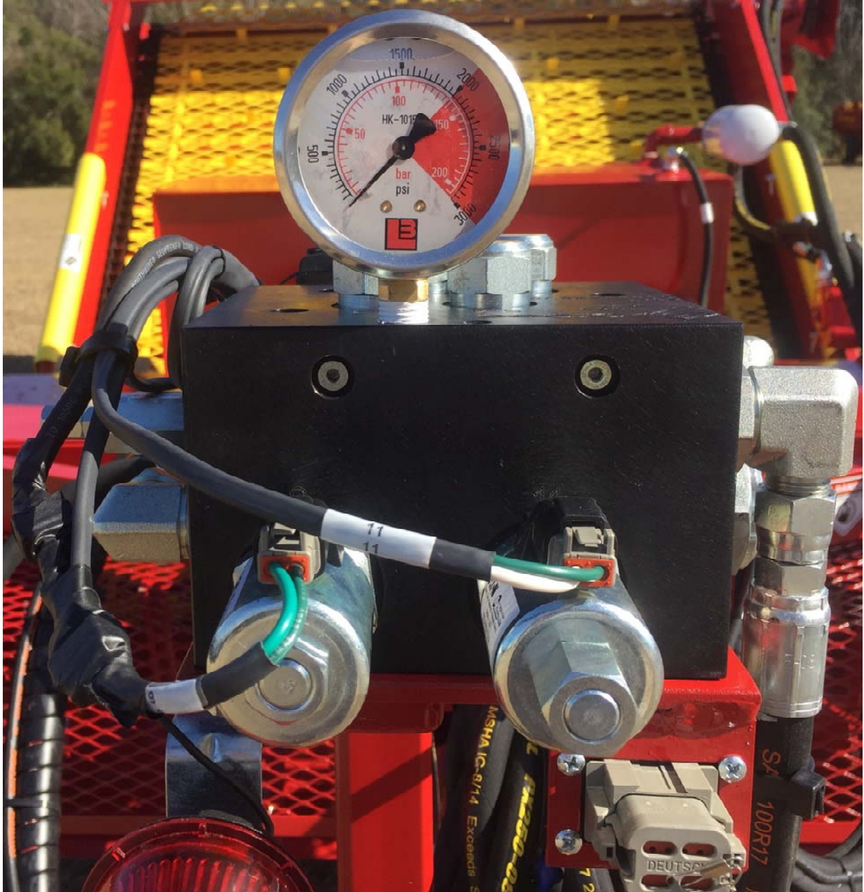
Electric Double Spool Valve Kit DB-400145
